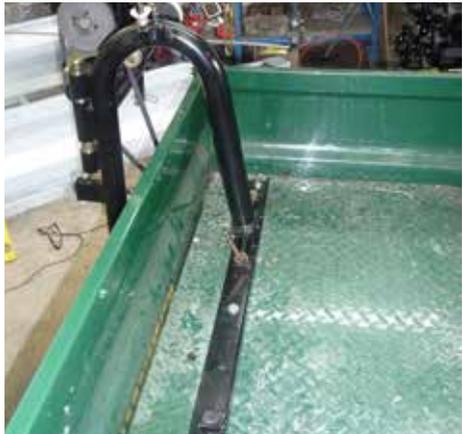
4. Connect the winder to the reel arm. Reel shafts should be at the top of the machine.
