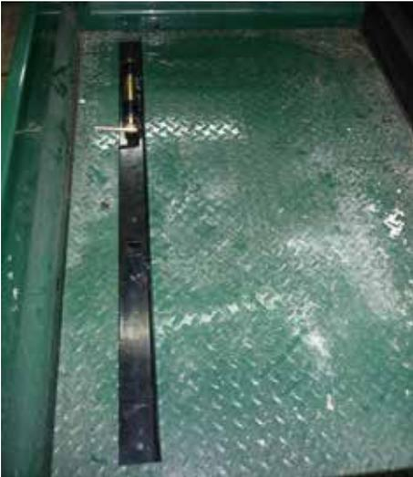
2. Connect the wheel arm to the mounting frame using the pin provided. The aim is to have the drive wheel sitting on the RTV wheel. The rear of the wheel arm frame should be at 90 degrees to the bed and slightly towards the outside of the RTV wheel. The actual position will vary depending on the make of the RTV. In some cases it may be necessary to move lights or mud flaps.
