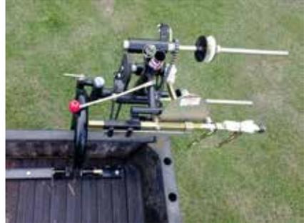
2. Slip the drive belt over Top Pulley and Wheel Arm Pulley twisting it to form a figure of eight.
